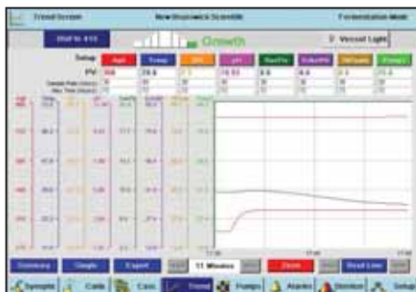
The trend graph screen makes it simple to track & export data on up to eight process variables over a six day span. Customize the view by selecting the parameters, colors & interval between sample measurements.
